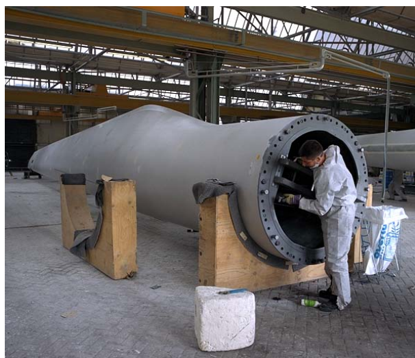
Figure 3: Blade under construction
